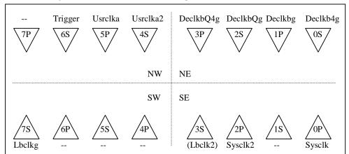
As much as possible, the User Core should only use the two main clocks **Lbclkg** and **Sysclk2**. The other clocks are used by the Agilent Acqiris-supplied cores.
