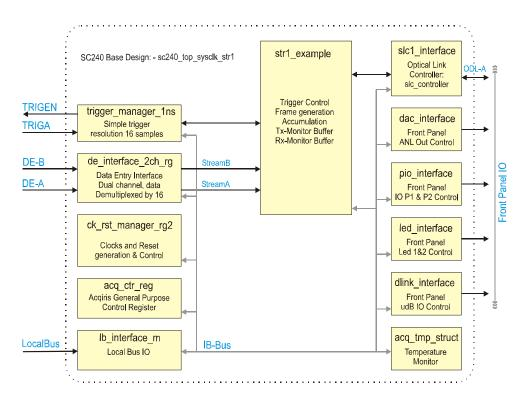
The streamer example block generates, manages, and sends three differents type of frames to the sfpdf controller **slc\_controller**: the raw data frame, the accumulated data frame, and the parameter data frame.
