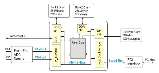
The Local Bus interface is entirely synchronous to the PCI clock, always running at 33 MHz.
