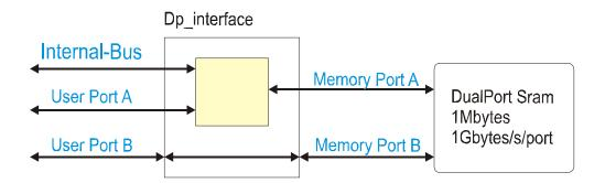
The dual port RAM can be read or written by the user program through the Internal Bus port. The Internal Bus port and the User port are multiplexed and cannot be used simultaneously. The Internal Bus port runs at 33 MHz. The priority of the Internal Bus over the User port is controlled by the bit **DPM\_Local** in the DP\_Control register.
