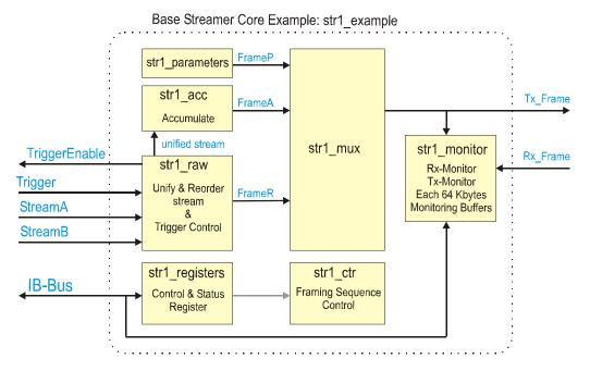
The block **str1\_raw** mixes the stream A and B to a single unified stream in an interleaved fashion. The unified stream could also be reordered in order to align the trigger position to the 16 samples data blocks. Once enabled and after each trigger, the block **str1\_raw** generates and sends a Raw Data frame to the FrameR port of the Frame multiplexer. The Raw Data frame has a 128 bits header followed by a programmable number of raw samples [or bytes].
