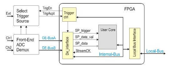
Once the acquisition is started, a continuous stream of data flows to the FPGA, along with the DE-Bus clocks **DECLKA** and **DECLKB**. Both are equal to the ADC clock, divided by 16.
