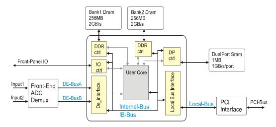
The analog input signals are passed through signal-conditioning amplifiers, where the coupling, offset, and gain can be programmed. Each signal is sampled at up to 1 GS/s and converted to 8-bit values. They are multiplexed to blocks of 16 samples, at up to 62.5 MHz, and passed to the data processing unit.
