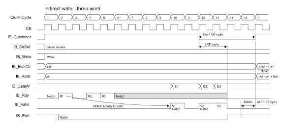
The delay Ready to Valid is due to the backward and forward pipelines within the Local Bus interface.
