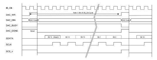
Note 1: Design limitation due to the use of IB\_Clk/2 to generate SCLK.
