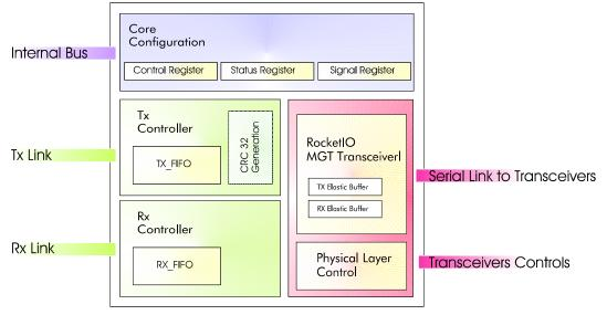
The figure hereafter presents a functional block diagram of the sFPDP Controller.
