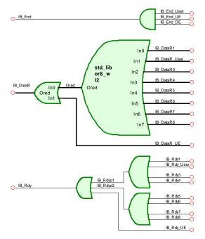
IB\_Rdy: The signal from all targets should be OR'd.
